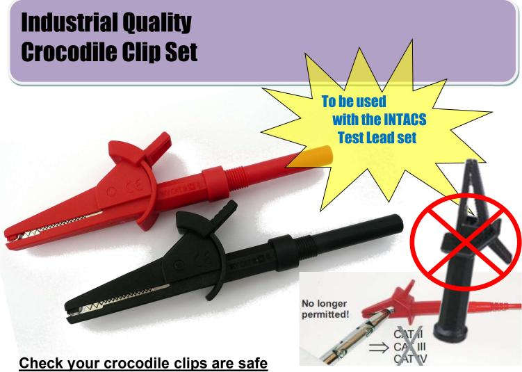
The International Standard for Test Equipment Accessories (IEC/EN 61010-031) informs that it **MUST NOT** be possible to touch any metal of the crocodile clip when in their closed state. This is particularly important with crocodile clips that employ the open jaw style if **CATII, CATIII or CATIV** rated. Please consider replacing with these safer type that INTACS stock.
